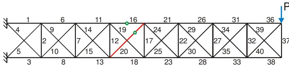
Fig. 5.1a Two sensors (dots) for precise identification of one damaged element No. 20
