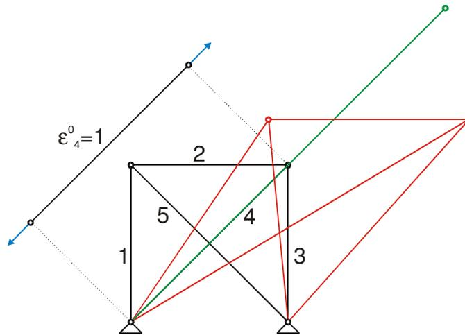
Fig. 2.1 Influence of the unit distortion applied in one element
