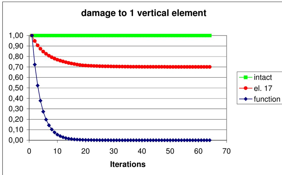
Fig. 5.3b Results of the identification process for 1 damage in a vertical member
