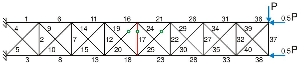
Fig. 5.3a Three sensors for precise identification of damage in one vertical element
