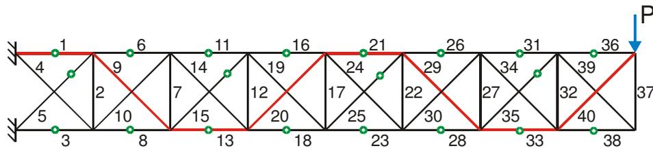
Fig. 5.2c Configuration of 20 sensors for identification of 8 damaged elements
